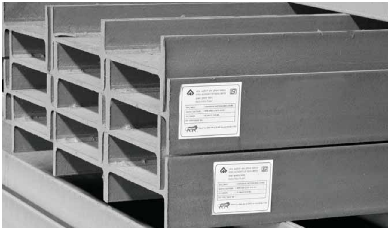
Narrow Parallel Flange Beam manufactured at Universal Section Mill at SAIL's IISCO Steel Plant.
