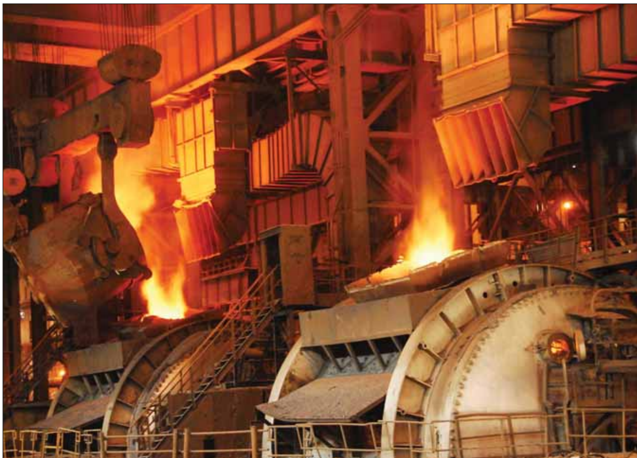
Hot Metal being poured into Mixer of Steel Melting Shop-II at SAIL's Rourkela Steel Plant.
